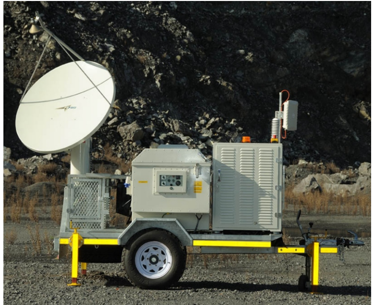
The MSR 300 - Movement and Surveying Radar
