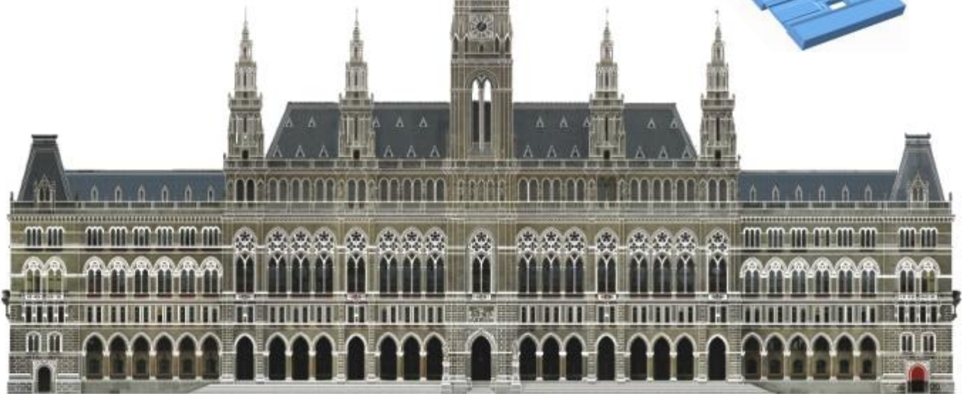
3D orthophoto computed out of 83 single scans and 88 digital images with an overall length of 155 metres and 98 metres in height.
